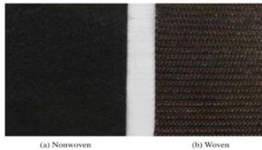
**Figure 3. Geotextile products**
