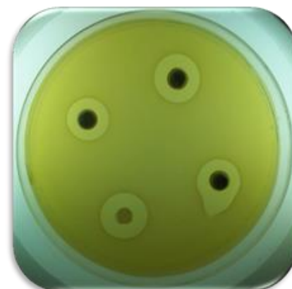
Figure: 4. Antimicrobial activity of a preparation of treated \text{TiO}_2 nano-composite composite with 10% (m/m) BzCl tested against E. faecalis . It is evident that the preparation possesses antimicrobial activity.
