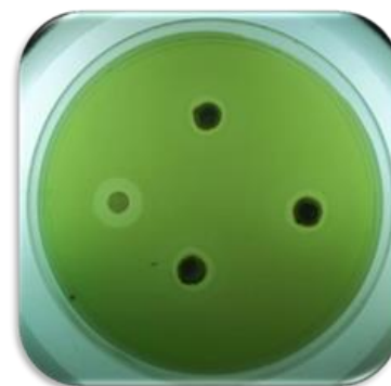
Figure: 5. Antimicrobial activity of a preparation of treated \text{TiO}_2 nano-composite composite with 10% (m/m) BzCl tested against P. aeruginosa . It is evident that the preparation possesses antimicrobial activity.
