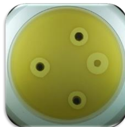
Figure: 3. Antimicrobial activity of a preparation of treated \text{TiO}_2 nano-composite composite with 10% (m/m) BzCl against E. coli . It is evident that the preparation possesses antimicrobial activity.
