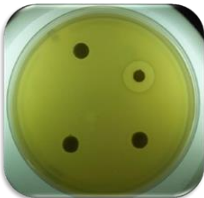
Figure: 1. Antimicrobial activity of untreated \text{TiO}_2 nano-composite tested against S. mutans . It is evident that the untreated \text{TiO}_2 does not possess antimicrobial activity.
