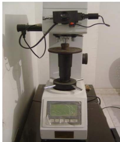
Figure 1. Digital Display Vickers Micro-hardness Tester Hardness were determined by the indentation technique. Three indentations were made on each specimen at widely separated locations with a load of 500 gram for 20 seconds in a micro hardness tester
