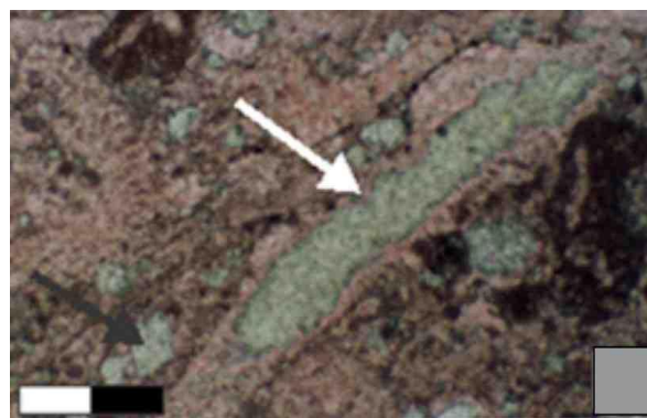
Figure 13. Photomicrograph of bioclastic dolomitic packstone (Verulam Formation). Note presence of chert replacing brachiopods (white arrow), and calcite cement, dolomite crystals of idiotopic type (black arrows). Scale bar is 240 Fm, sample 36m, Brechin quarry.
