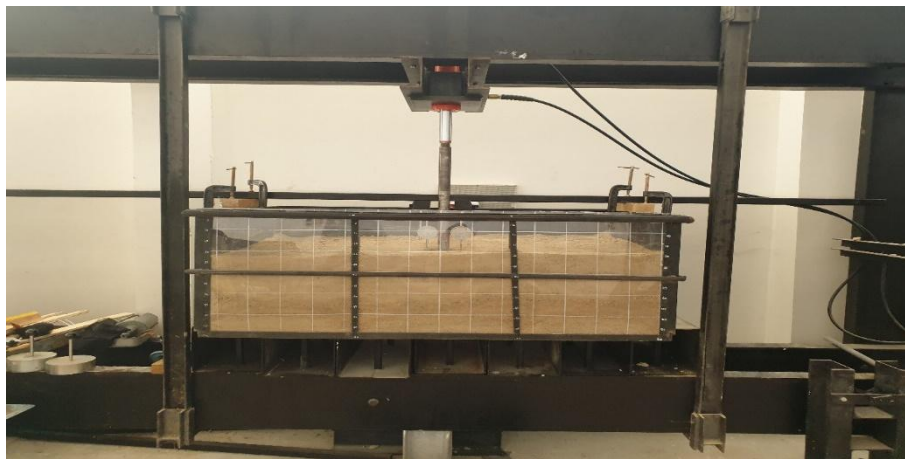
Figure 3. Model footing load test arrangement in the laboratory.
