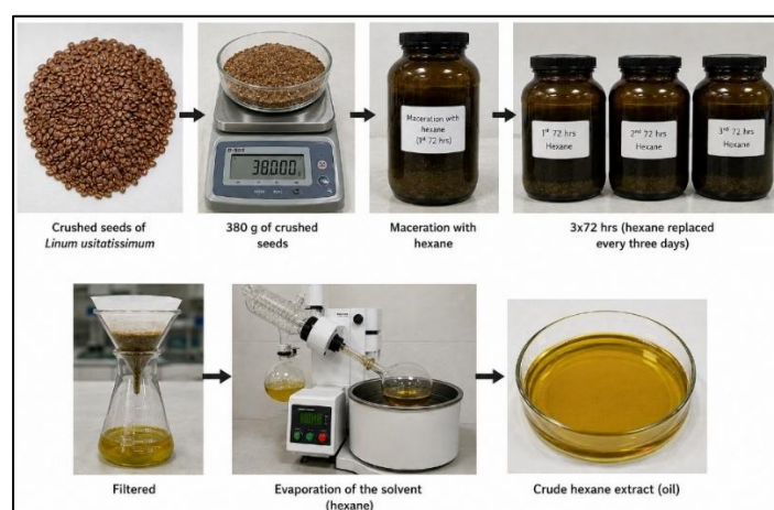
Figure 2. Hexane extraction of Linum usitatissimum seeds.
