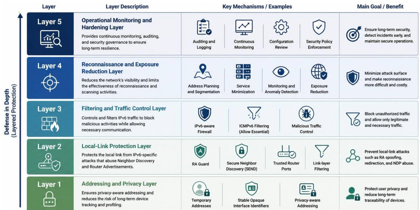
Figure 1. Proposed Layered IPv6 Security and Privacy Framework.
