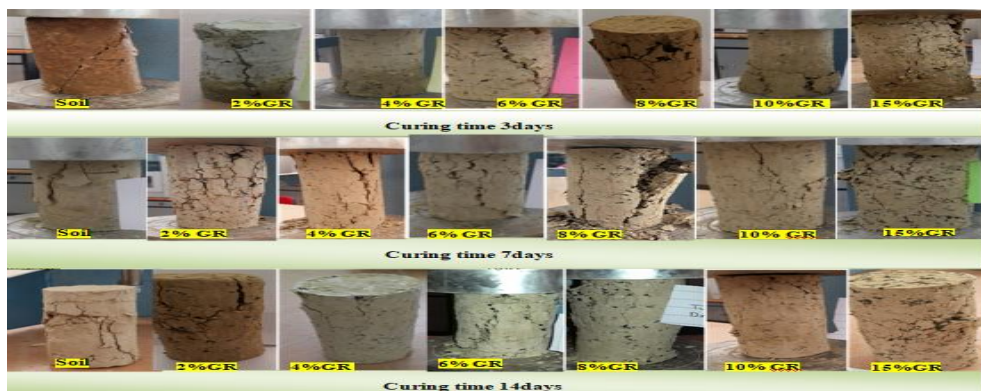
Figure 6. The shape of the failure of the samples
