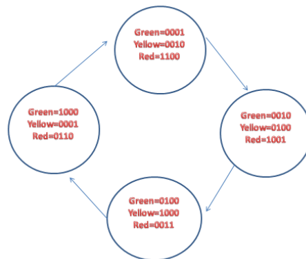
Figure 5. TLC State Diagram.
