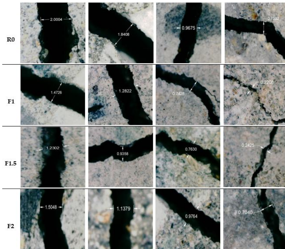
Fig. 7. The widest and narrowest crack widths of the samples due to the impact test
