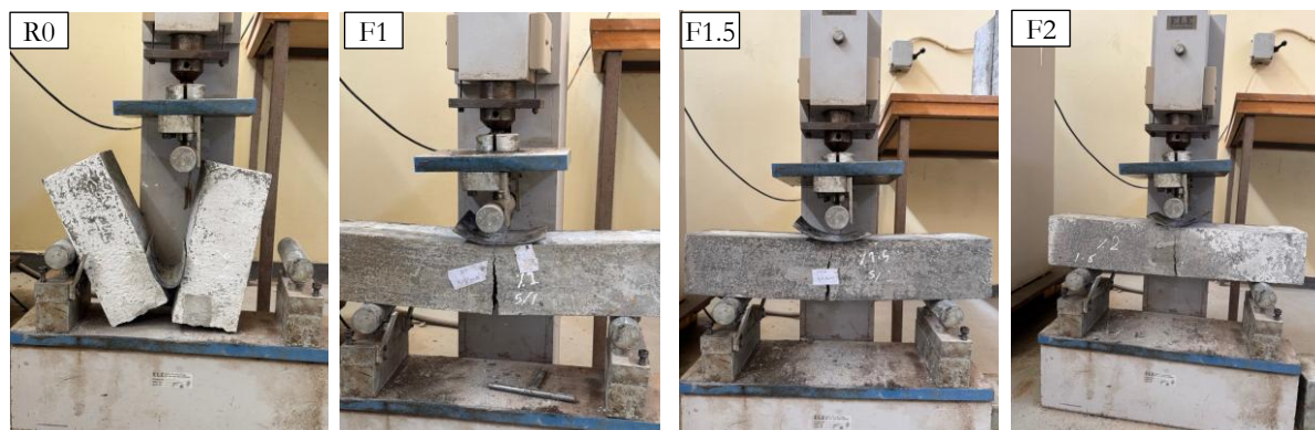
Fig. 8 Failure pattern of samples due to the flexural test
